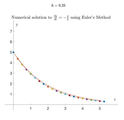
Unfortunately, small h means more iterations. Even more unfortunately, Euler's method is often not stable, meaning that the error in the approximation can quickly accumulate to such a size that the numerical solution diverges wildly from the true solution.
